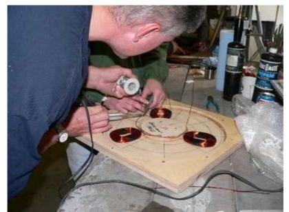
Wiring one phase of the stator.
