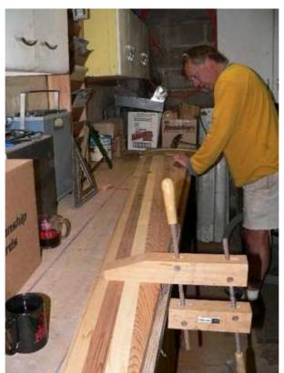
Clay from the MREA uses a mallet and chisel to remove the chunks that were kerfed with the bowsaw.
