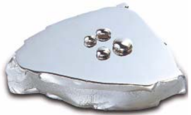
Fig. 1 A sample of Liquidmetal Technologies' Zr-based metallic glass.
