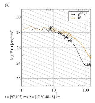
**Figure 16.** Energy spectra of the angular components of the velocity (black lines with stars) and magnetic field (orange lines with diamonds) in the PNS of Model B12 at  $t=100\,\mathrm{ms}$ . The energy spectra, E(l), are shown in comparison to the Kolmogorov scaling,  $l^{-5/3}$  (grey lines).
