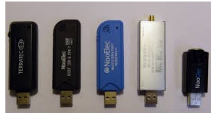
Terratec RS20T no TCXO Black NooElec RS20T no TCXO Blue NooElec RS20T2 TCXO Silver dongle RS20T2 TCXO Nano NooElec RS20T no TCXO
