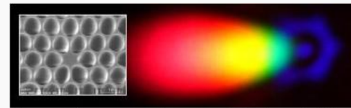
Supercontinuum generation using photonic crystal fibers
