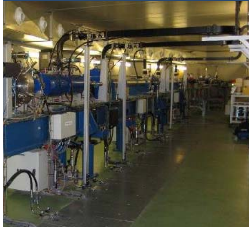
LINAC: 3GHz structure, beam acceleration to 100 MeV
