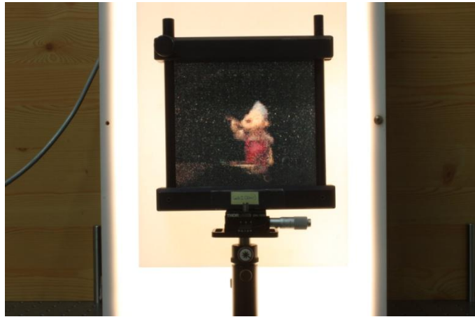
Fig. 11. Experimental setup for the observation of the hexagonal InI monitor. After displacing horizontally the camera in steps of 10 mm, we recorded 35 different perspectives of the displayed 3D scene.
