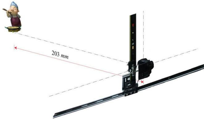
Fig. 3. Scheme of the experimental set up for the acquisition of the set of elemental images of a 3D scene.
