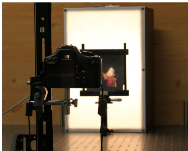
Fig. 7. Experimental setup for the observation of the InI monitor. After displacing horizontally the camera in steps of 10 mm we recorded 20 different perspectives of the displayed 3D scene.
