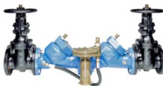
Fig. 25. A reduced-pressure-type backflow preventer contains two check valves with a relief valve located in between them (Source: https://www.labdesignnews.com/article/2010/04/understanding-laboratory-plumbing-systems-water )
