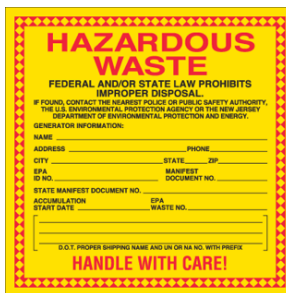
Fig. 12. Example of contents for an External hazardous waste label (Source: Environmental Protection Agency (EPA))
