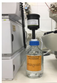
Fig. 31. Example of safety caps for VOCs bottles (Source: Provided by a participant laboratory)
