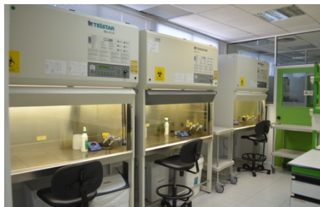
Fig. 30. Biosafety cabinets class II with laminar flow technology (Source: Provided by a participant laboratory)
