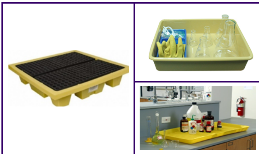
Fig. 7. Examples of anti-spill containers (Source: Provided by a participant laboratory and https://www.calpaclab.com/storage-totes-and-trays/ )
