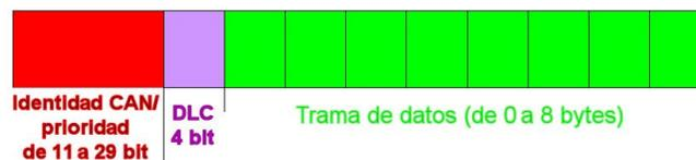
Figura 22. Formato de trama CAN (DLC = Data Length Code).
