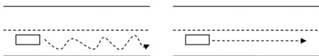
Fig. 4 Two trajectories of car with values of TLC close to zero (left) or infinite (right)
