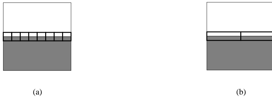
Fig. 2. A simple image with one linear horizontal discontinuity is represented by the two types of basis functions. (a) Isotropic basis functions generate a large number of significant coefficients around the discontinuity. (b) Anisotropic basis functions trace the discontinuity line and produce just a few significant coefficients.
