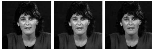
Figure 13: Three different frames from Miss America sequence using the adaptive compression system. The first three are at next simulation transitions: switch from 10 to 5 Mbps, switch from 5 to 2 Mbps and finally at 2 Mbps
