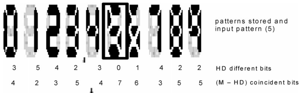
Figure 2. The stored patterns consist of seven black and white segments that represent a number (see Yamanaka et al. 2 ). The black or white state of each segment corresponds to a bit, and the numbers are represented by N = 10 vectors, each one with M = 7 binary elements. The Hamming distance (HD) is the number of different bits between the input pattern (the number 5 within the square) and each of the 10 stored patterns.
