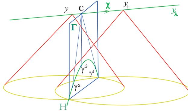
**FIGURE 2.** A time-like configuration ( $\chi^2 < 0$ ). There are two distinct points having the same emission coordinates but different Cartesian representation,  $y_+$  and  $y_-$ , respectively. Both roots of the quadratic equation provide emission solutions. The straight line  $y_\lambda$  is space-like and cut the time-like hyperplane  $\Gamma$  at the event  $C$ , which is the center of a space-like 2-hyperboloid  $\mathbb{H}$  containing these four configuration events.
