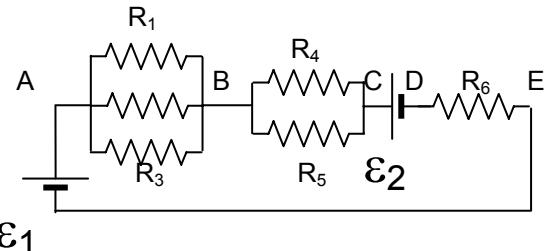
SOL:  $I = 0.2 \text{ A}$ ,  $V_A - V_B = 2 \text{ V}$ ,  $V_B - V_C = 1.6 \text{ V}$ ,
