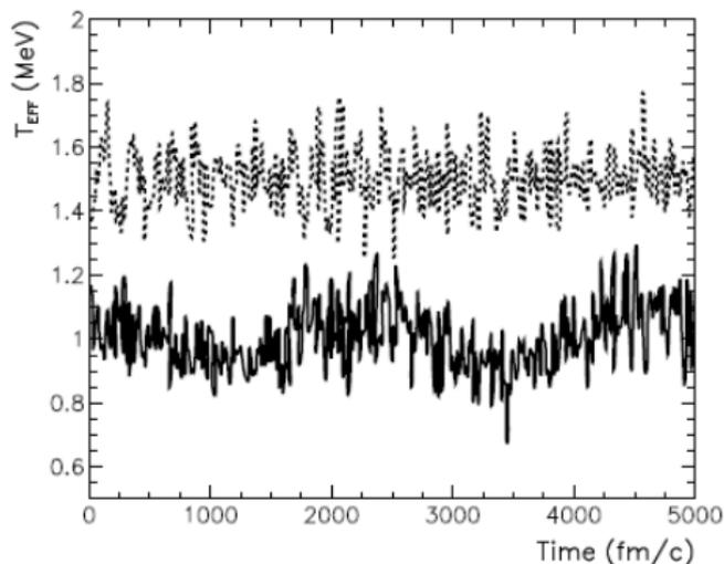
Thermal bath: better  $T$  control in the NVT system than rescaling
