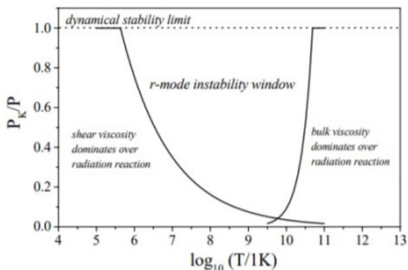
Fig. 3. The critical rotation rates at which shear viscosity (at low temperatures) and bulk viscosity (at high temperatures) balance gravitational radiation reaction due to the  $r$ -mode current multipole. This leads to the notion of a “window” in which the  $r$ -mode instability is active. The data in the figure is for the  $l = m = 2$   $r$ -mode of a canonical neutron star ( $R = 10$  km and  $M = 1.4M_{\odot}$  and Kepler period  $P_K \approx 0.8$  ms).
