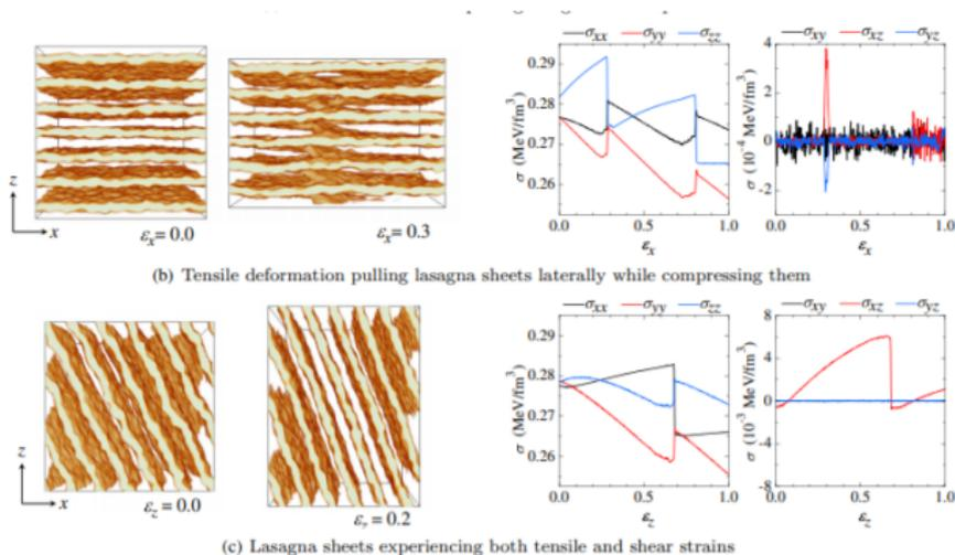
Pasta max. breaking strains of order  $0.1 \text{ MeV}/\text{fm}^3$ .  $n_b = 0.05 \text{ fm}^{-3}$ ,
