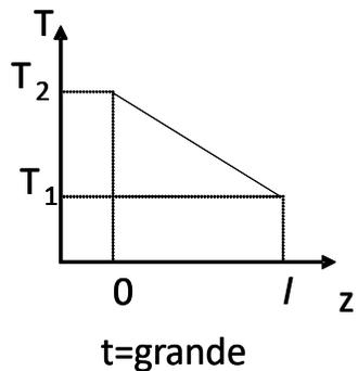
$$\frac{dT}{dz} = \frac{\Delta T}{\Delta z} = \frac{T_2 - T_1}{z_2 - z_1} = \frac{275 - 325}{200} = -0.25 \text{K} \cdot \text{cm}^{-1}$$
