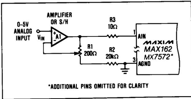
Figure 18. Full-Scale Adjustment
