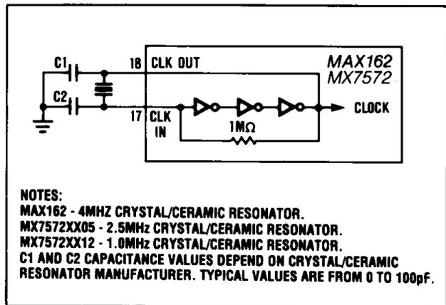
Figure 6. MAX162/MX7572 Internal Clock Circuit
