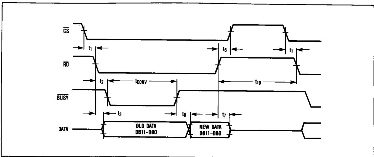
Figure 10. Slow Memory Mode, Parallel Read Timing Diagram
