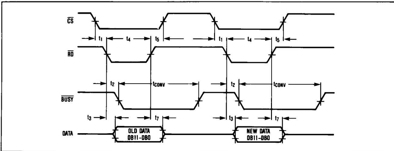
Figure 12. ROM Mode, Parallel Read Timing Diagram
