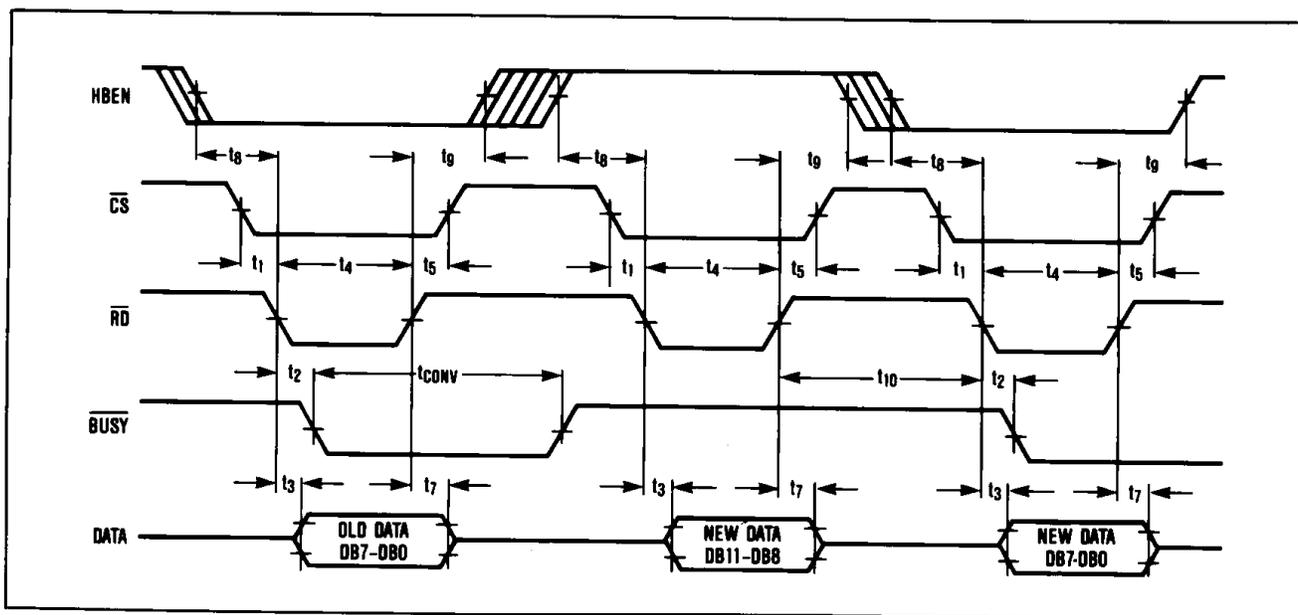
Figure 13. ROM Mode, Two Byte Read Timing Diagram
