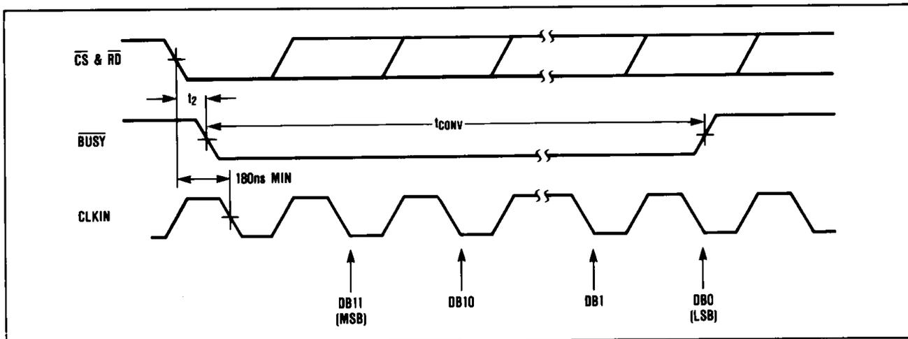
Figure 8. MX7572  $\overline{RD}$  and CLKIN For Synchronous Operation
