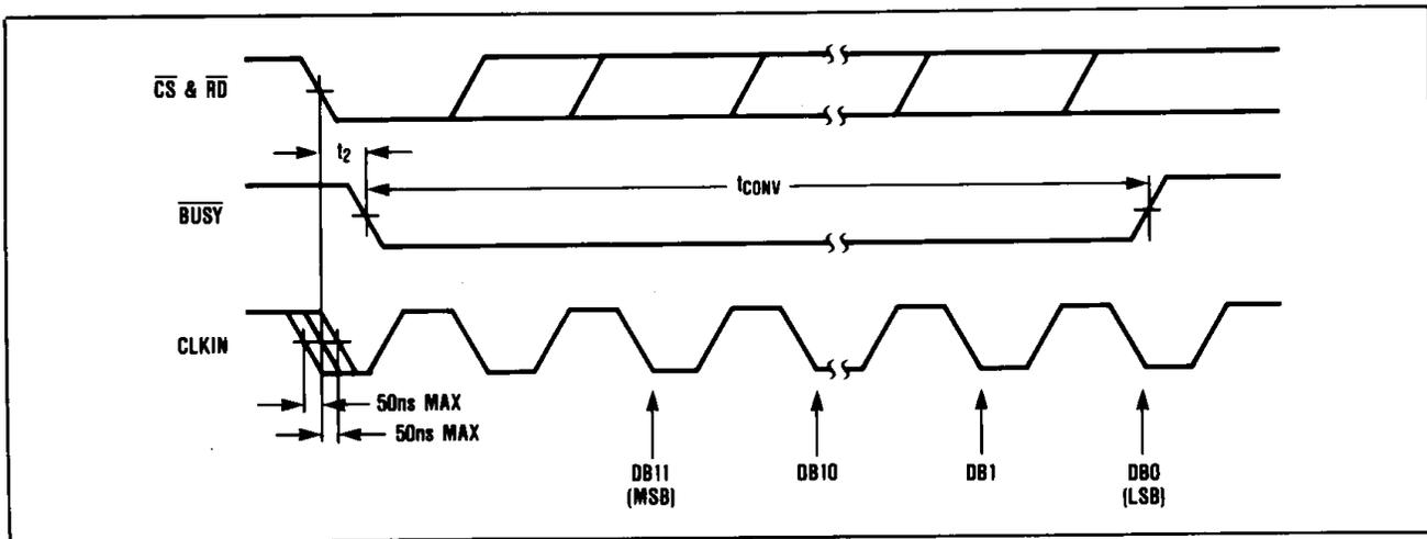
Figure 7. MAX162  $\overline{RD}$  and CLKIN For Synchronous Operation
