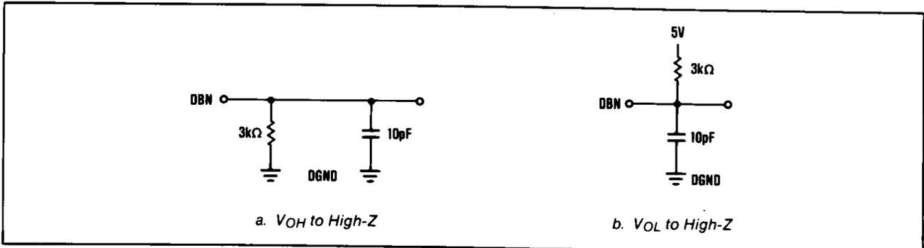
Figure 2. Load Circuits for Output Float Delay
