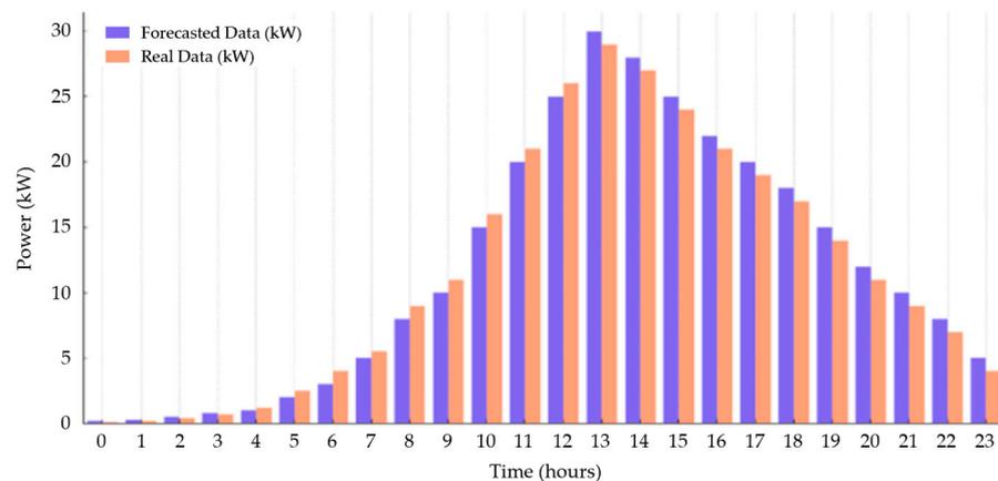
**Figure 2.** 24-h charging load profile: forecast accuracy assessment. Blue bars represent “Forecasted Data”, and orange bars represent “Real Data”.
