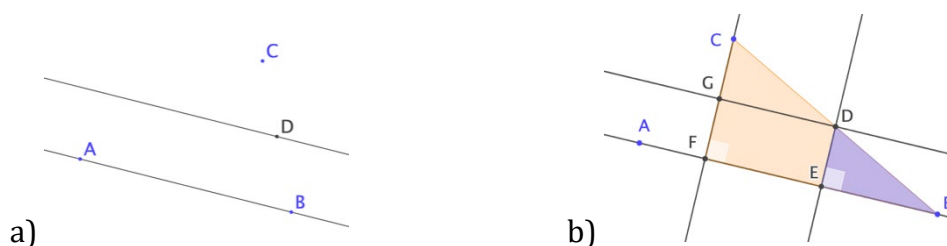
Figure 1. Construction of equidistant line from three non-collinear points in 2D configuration.
