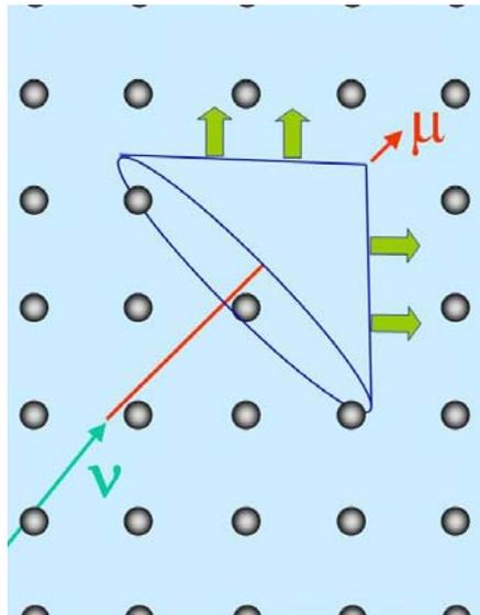
**Figure 5.11:** Neutrino telescopes consist of large arrays of photomultiplier tubes underwater or under ice. They detect the Cherenkov light emitted by charged particles which have been produced in neutrino interactions – here from an up-going muon which stems from a neutrino having crossed the Earth.
