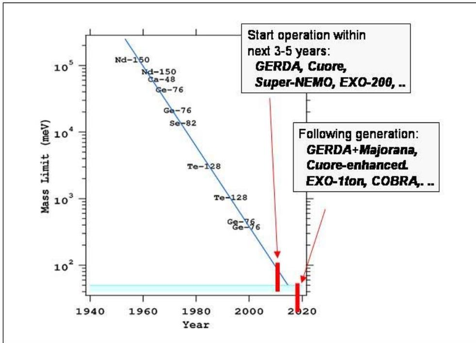
*Figure 3.7: A possible scenario for improvement of the mass sensitivity of double beta experiments (figure adopted from Elliot and Vogel).*
