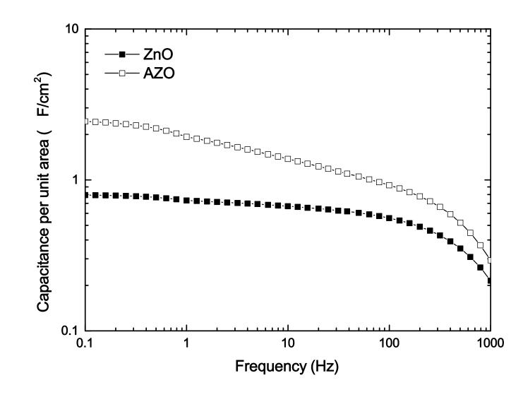
Capacitance as a function of frequency for the ZnO and
