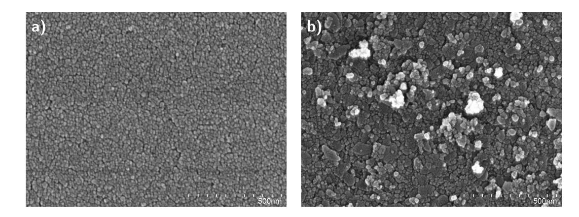
SEM images of the a) ZnO and b) AZO nanoparticles layer after the annealing (120 minutes, 150 °C).
