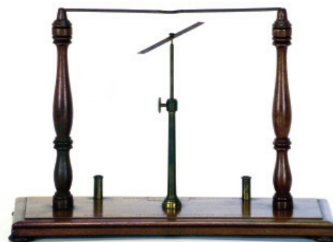
Agulha de Oersted, E.M. Clarke, a.1851. (Foto: acervo GF/UC)
