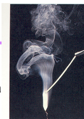
FIGURE 3.10 Metallic magnesium burns in air. The reaction produces a large amount of heat and light. The product of the reaction, magnesium oxide, can be seen dangling from the burning magnesium ribbon.
