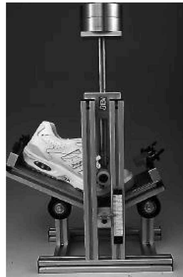
Fig. 4. Machine to determine transverse flexibility (flexion).
