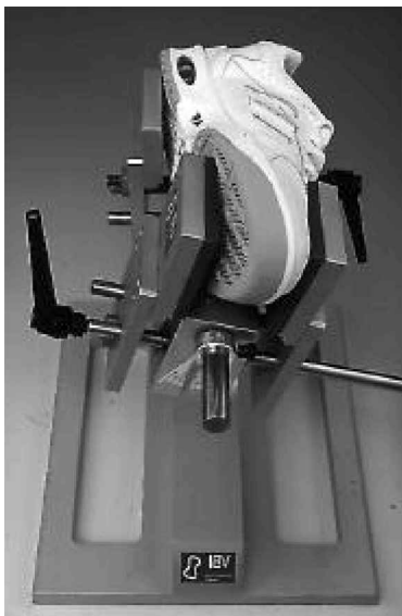
Fig. 3. Machine to determine longitudinal flexibility (torsion).
