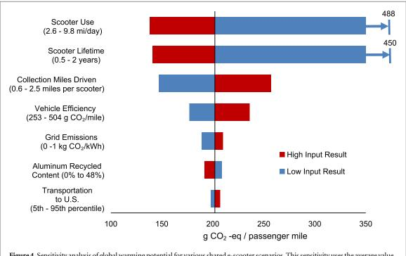
Figure 4. Sensitivity analysis of global warming potential for various shared e-scooter scenarios. This sensitivity uses the average value from the base case scenario as seen previously in figure 3, but applies a static low and high value to the input parameter of interest shown in parentheses along the y axis.
