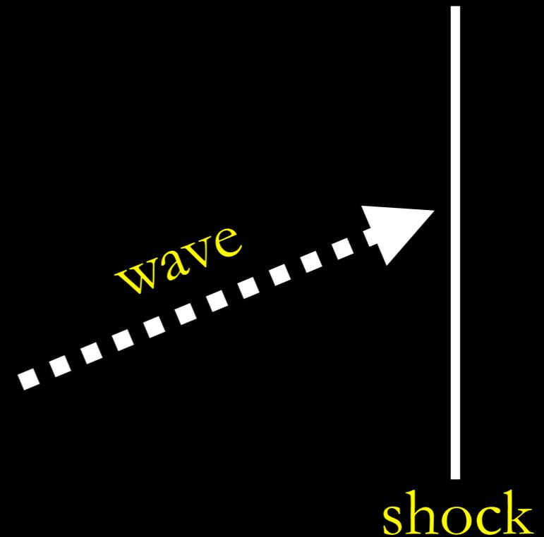
**Method: decompose turbulence into waves, calculate interaction for each wave, and integrate the result over all waves**
