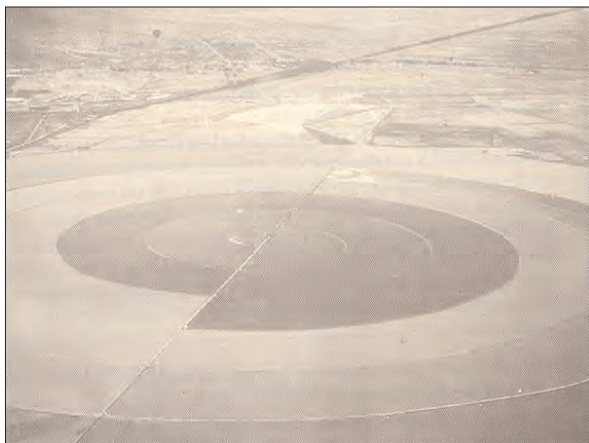
Figure 3. The “snail”. An enormous solar evaporator (its diameter is 3.4 km) constructed for the Texcoco-valley-subterranean-waters’ concentration of salts, in the industry “Sosa Texcoco”, founded in 1943.
