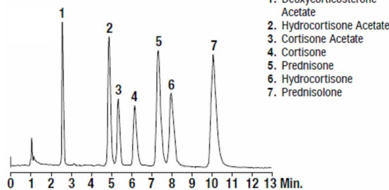
**Column:** Alltech® Alltima™ HP CN, 5 $\mu$ m, 150 x 4.6mm
