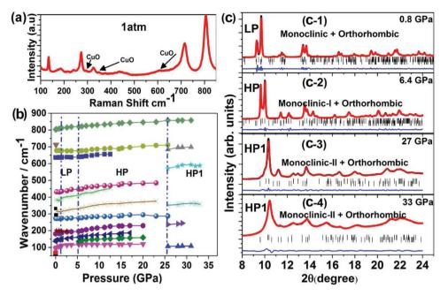
**Figure 4.** a) Raman spectra of  $WO_3/CuO$  at ambient conditions where the CuO nanoparticles contributions were confirmed. The corresponding modes related to  $WO_3$  and CuO are marked. b) The variation of the Raman active modes of  $WO_3/CuO$  under compression up to 37 GPa. c) The XRD patterns with Rietveld refinements and different phase coexistence are shown at a few representative pressure points. For simplicity, LP, HP, and HP1 are marked for different pressure regions (see text).
