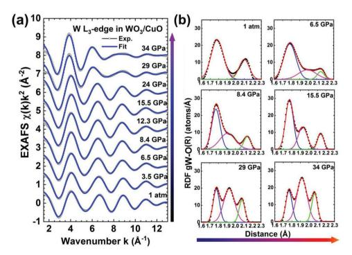
**Figure 5.** a) The pressure dependence of the experimental and calculated W L<sub>3</sub>-edge EXAFS for the first coordination shell of tungsten. b) Decomposition of the RDFs  $g_{W-O}(R)$  (solid circles) for the first coordination shell of tungsten into Gaussian components (solid lines). A variation of the WO<sub>6</sub> octahedra distortion upon compression is well observed.
