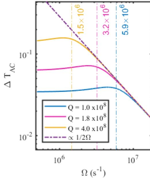
Fig. 3: Frequency response of the dynamically modulated optical ring resonator.
