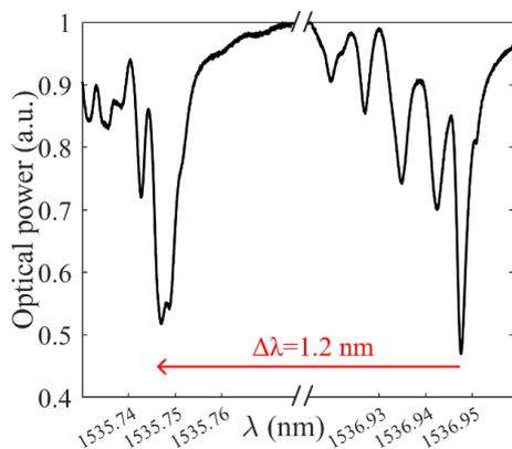
Fig. 3: Wavelength shift of a TM-WGMR when it is measured in the pristine (right) and the UV-irradiated (left) section of the MR.
