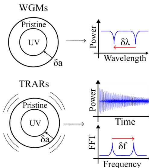
Fig. 1: Principle of operation of the (up) WGMRs technique, (low) TRARs technique.
