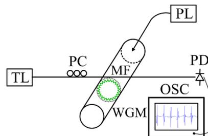
Fig. 4: Scheme of the setup for the TRARs technique. PL: high peak power pump laser.
