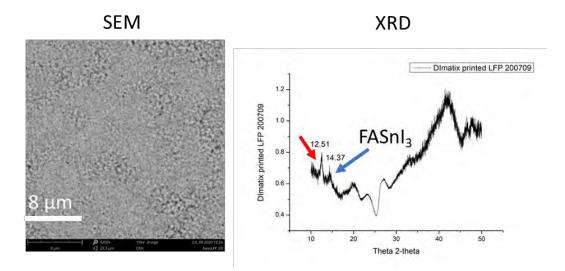
**Figure 2.** Inkjet printed FASnI<sub>3</sub> thin film in ambient conditions and crystallized using vacuum assisted annealing process on a flexible PET/ITO/PEDOT:PSS substrate: (left) SEM image and (right) XRD pattern. Blue arrow indicates the diffraction peak of the (100) plane for FASnI<sub>3</sub>, while the red arrow indicates the signal from some byproduct.
