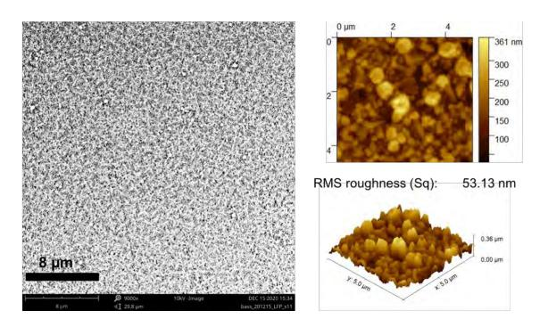
**Figure 4.** (left) SEM image of inkjet printed Ag<sub>3</sub>Bil<sub>6</sub> thin film. (right) 2D and 3D AFM topography images of printed Ag<sub>3</sub>Bil<sub>6</sub> thin film.
