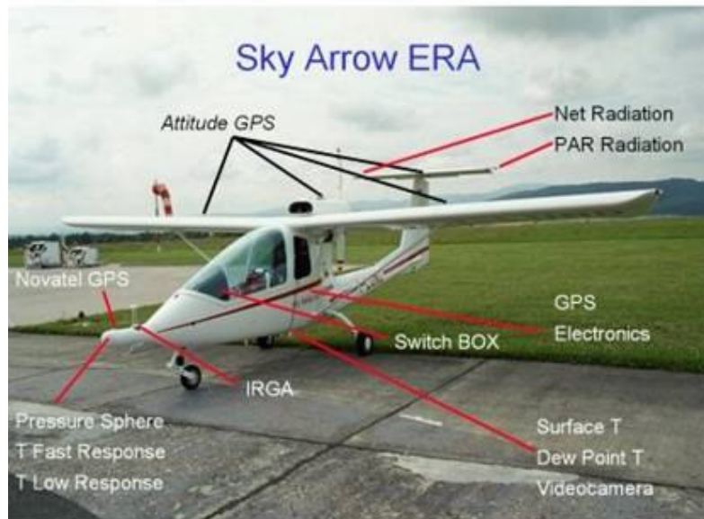
Figure 9. Flux airplane with instruments mounted on board
