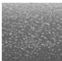
Surface of an optical fiber decorated with mesoporous silica nanoparticles
