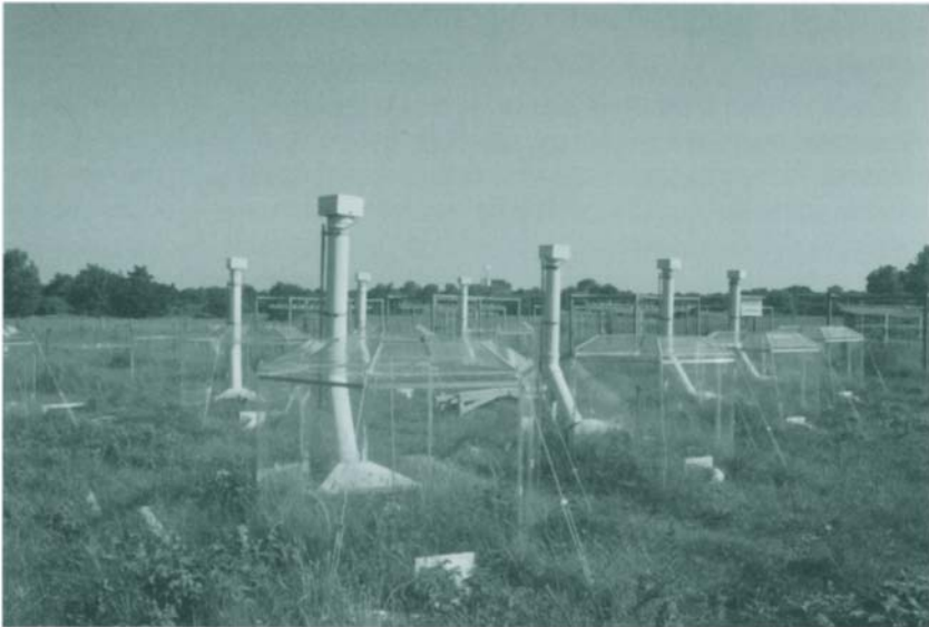
Figure 4 Open top chambers for CO 2 enrichment (foreground) and UV-fluorescent tubes (background) for a UV-B supplementation system in the dune grassland in Heemskerk, The Netherlands. (Photograph courtesy of J. Rozema.)
