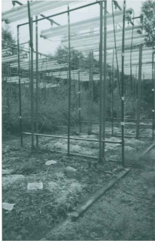
Figure 7 Litter bags filled with senesced leaves of Holcus lanatus exposed to ambient or enhanced UV-B at an experimental field at the campus of the Vrije Universiteit, Amsterdam, The Netherlands. Litter bags are on the soil surface without vegetation to assess photodegradative effects of UV-B on the rate of mass loss of litter. Philips TL 12/40 fluorescent tubes have been installed in racks at a height of 1.40 m above the soil surface. Both for ambient UV-B and for enhanced UV-B, the fluorescent tubes were operating, but they have different filters to effect the appropriate UV-B supplementation levels. The enhanced UV-B treatment was designed to simulate about 15% stratospheric ozone depletion at this site. In this design, the ambient and enhanced UV-B treatment had the same flux of UV-A radiation. Litter in the litter bags originates from Holcus lanatus plants exposed to ambient ( 5 \text{ kJ m}^{-2}\text{d}^{-1} ) or enhanced ( 7.5 \text{ kJ m}^{-2}\text{d}^{-1} UV-B BE ) for one growing season (Photograph courtesy of J. Rozema.)
