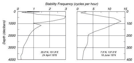
Figure 8.5. Observed stratification frequency in the Pacific. **Left:** Stability of the deep thermocline east of the Kuroshio. **Right:** Stability of a shallow thermocline typical of the tropics. Note the change of scales.
