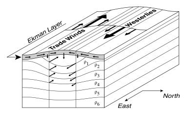
Figure 12.6 Winds at the sea surface drive Ekman transports to the right of the wind in this northern hemisphere example (bold arrows in shaded Ekman layer). The converging Ekman transports driven by the trades and westerlies drives a downward geostrophic flow just below the Ekman layer (bold vertical arrors), leading to downward bowing constant density surfaces  $\rho_i$ . Geostrophic currents associated with the warm water are shown by bold arrows. (After Tolmazin, 1985)
