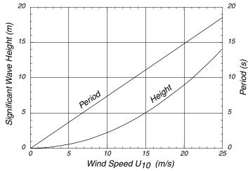
Figure 16.8 Significant wave height and period at the peak of the spectrum of a fully developed sea calculated from the Pierson-Moskowitz spectrum using (16.15 and 16.32).
