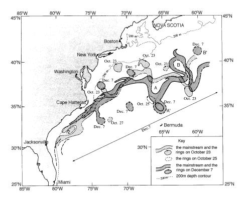
Figure 11.12 Sketch of the position of the Gulf Stream, warm core, and cold core eddies observed im infrared images of the sea surface collected by the infrared radiometer on NOAA-5 in October and December 1978 (from Tolmazin, 1985: 91).
