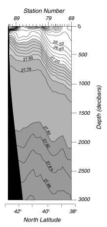
Figure 10.12 Cross section of potential density  $\sigma_{\theta}$  across the Gulf Stream along 63.66°W calculated from CTD data collected from *Endeavor* on 25–28 April 1986. The Gulf Stream is centered on the steeply sloping contours shallower than 1000m between 40° and 41°. Notice that the vertical scale is 425 times the horizontal scale. (Data contoured by Lynn Talley, Scripps Institution of Oceanography).
