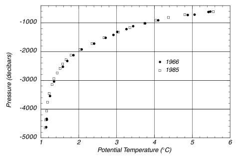
Figure 8.8 Potential temperature measured as a function of depth (pressure) near 24.7°N, 161.4°W in the central North Pacific by the *Yaquina* in 1966 ( $\bullet$ ), and by the *Thompson* in 1985 ( $\square$ ). Data from *Atlas of Ocean Sections* produced by Swift, Rhines, and Schlitzer.
