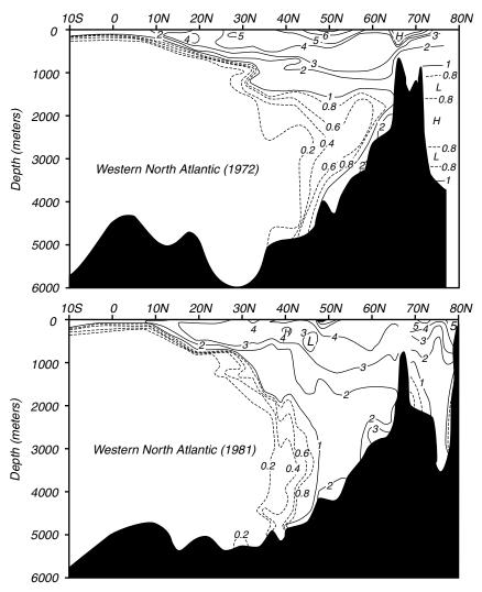
Figure 10.16 Distribution of tritium along a section through the western basins in the North Atlantic, measured in 1972 ( $\mathbf{Top}$ ) and remeasured in 1981 ( $\mathbf{Bottom}$ ). Units are tritium units, where one tritium unit is  $10^{18}$  (tritium atoms)/(hydrogen atoms) corrected to the activity levels that would have been observed on 1 January 1981. Compare this figure to the density in the ocean shown in Figure 13.9. From Toggweiler (1994)
