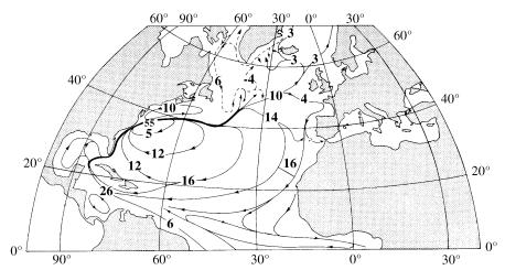
Figure 11.8 Schematic of currents in the North Atlantic showing major surface currents. Values are transport in units of  $10^6$  m<sup>3</sup>/s (From Sverdrup, Johnson, and Fleming 1942: Fig. 187).
