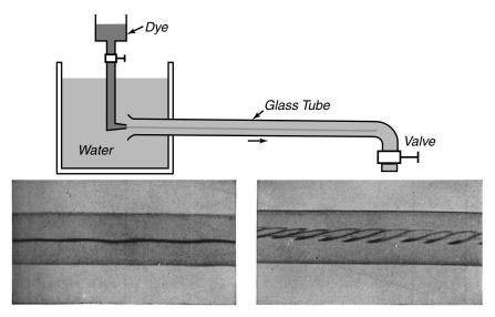
Figure 8.2 **Upper:** Reynolds apparatus for investigating the transition to turbulence in pipe flow. **Lower:** Photographs of near-laminar flow (left) and turbulent flow (right) in a clear pipe much like the one used by Reynolds. (From Binder 1953).
