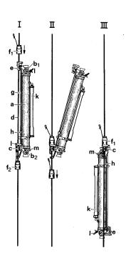
Figure 6.18 Left A CTD ready to be lowered over the side of a ship (From Davis, 1987). Right Nansen water bottles before (I), during (II), and after (III) reversing. Both instruments are shown at close to the same scale (From Dietrich et al. 1980).
