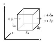
Figure 7.6 Sketch of flow used for deriving the continuity equation.
