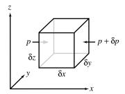
Figure 7.4 Sketch of flow used for deriving the pressure term in the momentum equation.
