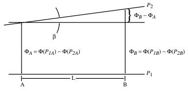
Figure 10.7. Sketch of geometry used for calculating geostrophic current from hydrography.
