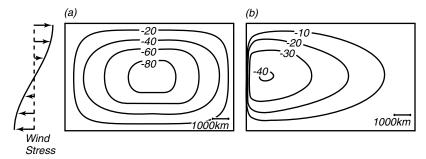
Figure 11.5 Stream function for flow in a basin as calculated by Stommel (1948). **Left:** Flow for non-rotating basin or flow for a basin with constant rotation. **Right:** Flow when rotation varies linearly with y.
