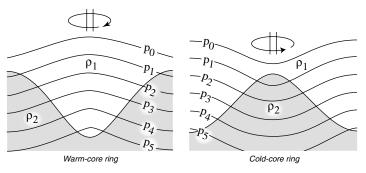
Figure 10.13 Shape of isobaric surfaces  $p_i$  and the interface between two water masses of density  $\rho_1, \rho_2$  if the upper is rotating faster than the lower. **Left:** Anticylconic motion, warm-core eddy. **Right:** Cyclonic, cold-core eddy. Note that the sea surface  $p_0$  slopes up toward the center of the warm-core ring, and the isopycnal surfaces slope down toward the center (From Defant, 1929).
