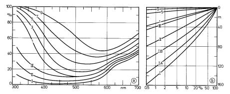
Figure 6.20 **Left:** Attenuation of daylight in the ocean in % per meter as a function of wavelength. I: extremely pure ocean water; II: turbid tropical-subtropical water; III: mid-latitude water; 1-9: coastal waters of increasing turbidity. Incidence angle is 90° for the first three cases, 45° for the other cases. (From Jerlov, 1951). **Right:** Percentage of 465 nm light reaching indicated depths for the same types of water. (From Jerlov, 1968).
