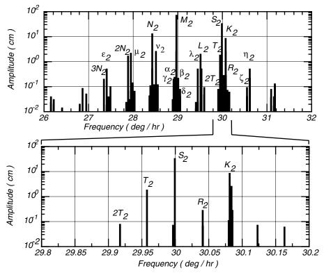
Figure 17.13 **Upper:** Spectrum of equilibrium tides with frequencies near twice per day. The spectra is split into groups separated by a cycle per month (1 deg/hr). **(Lower:** Expanded spectra of the  $S_2$  group, showing splitting at a cycle per year (0.04 deg/hr). The finest splitting is at a cycle per 8.847 years (0.0046 deg/hr).
