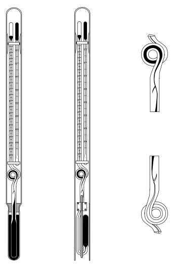
Figure 6.13 Left: Protected and unprotected reversing thermometers is set position, before reversal. Right: The constricted part of the capillary in set and reversed positions (From von Arx, 1962).
