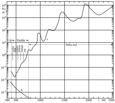
Figure 6.19 Attenuation coefficient c and scattering coefficient b for pure water as a function of wavelength  $\lambda$  of the radiation (From Dietrich, et al. 1980).
