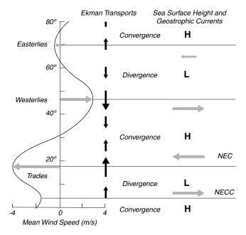
Figure 12.8 An example of how winds produce geostrophic currents running upwind. Ekman transports due to winds in the north Pacific (**Left**) lead to Ekman pumping (**Center**), which sets up north-south pressure gradients in the upper ocean. The pressure gradients are balanced by the Coriolis force due to east-west geostrophic currents (**Right**). Horizontal lines indicate regions where the curl of the zonal wind stress changes sign.
