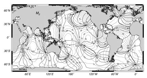
Figure 17.14 Global map of  $M_2$  tide calculated from Topex/Poseidon observations of the height of the sea surface combined with the response method for extracting tidal information. Full lines are contours of constant tidal phase, contour interval is 30°. Dashed lines are lines of constant ampliture, contour interval is 10 cm. (From Richard Ray, NASA Goddard Space Flight Center).
