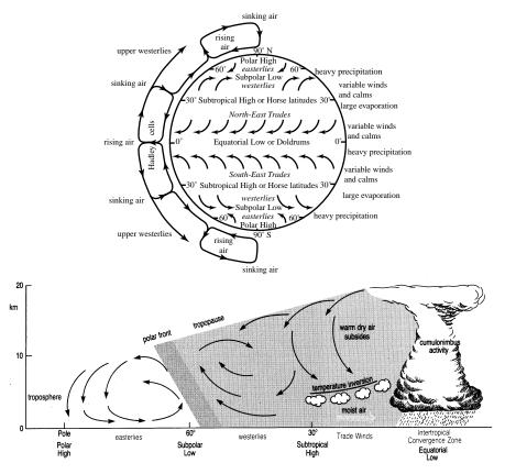
Figure 4.3 Simplified schematic of Earth's atmospheric circulation driven by solar heating in the tropics and cooling at high latitudes. **Upper:** The meridional cells in the atmosphere and the influence of Earth's rotation on the winds. **Bottom:** Cross-section through the atmosphere showing the two major cells of meridional circulation. From The Open University (1989a).
