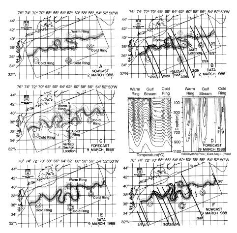
Figure 15.5 Output from the Harvard Open-Ocean Model: (Top) Data used for initializing the model on 2 March 1988 and the initial state of the model, the nowcast. (Center) The forecast for 9 March 1988. (Lower) The data used for determining currents on 9 March 1988 and the state of the ocean on that date calculated by the model using the new data. Although the Gulf Stream changed substantially in one week, the model forecasts the changes well. (From Robinson et al. 1989)
