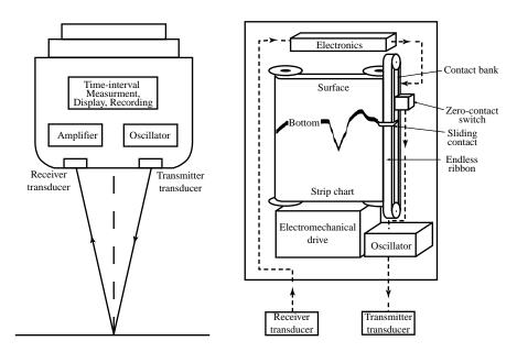
Figure 3.10 Left: Echo sounders measure depth of the ocean by transmitting pulses of sound and observing the time required to receive the echo from the bottom. Right: The time is recorded by a spark burning a mark on a slowly moving roll of paper. (From Dietrich, et al. 1980)
