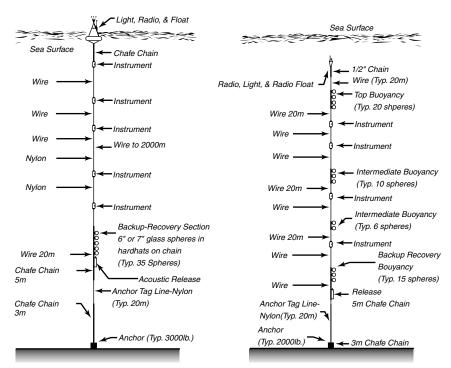
Figure 10.19 **Left:** An example of a surface mooring of the type deployed by the Woods Hole Oceanographic Institution's Buoy Group. **Right:** An example of a subsurface mooring deployed by the same group. (From Baker, 1981).
