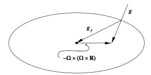
Figure 7.5 Downward acceleration g of a body at rest on Earth's surface is the sum of gravitational acceleration between the body and Earth's mass  $g_f$  and the centrifugal acceleration due to Earth's rotation  $\Omega \times (\Omega \times R)$ . The surface of an ocean at rest must be perpendicular to g, and such a surface is close to an ellipsoid of rotation. Earth's ellipticity is greatly exaggerated here.
