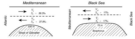
Figure 7.2 Schematic diagram of the flow in and out of: **left:** a salty sea, the Mediterranean Sea; and **right:** a fresher sea, the Black Sea. From Pickard and Emery, 1990.
