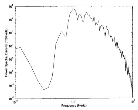
Figure 16.6 The spectrum of waves calculated from 11 minutes of data shown in Figure 7.2 by averaging four periodograms to reduce uncertainty in the spectral values. Spectral values below  $0.04~\mathrm{Hz}$  are in error due to noise.
