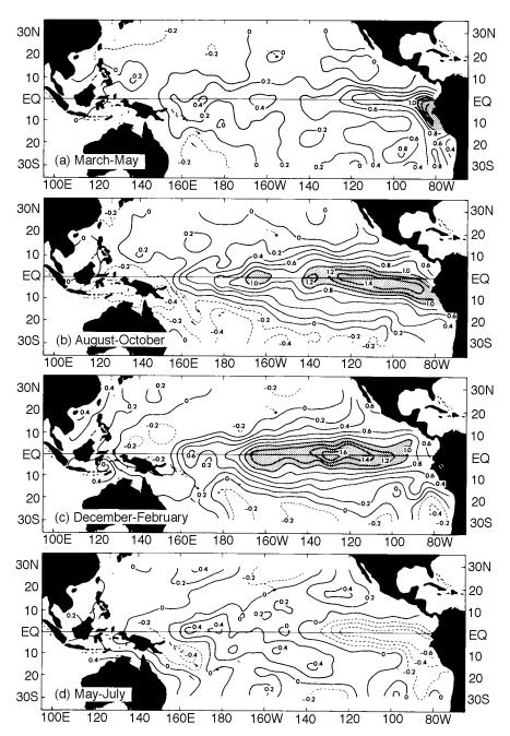
Figure 14.8 Anomalies of sea-surface temperature (in  $^{\circ}$ C) during a typical El Niño obtained by averaging data from El Niños between 1950 and 1973. Months are after the onset of the event. (From Rasmusson and Carpenter, 1982).
