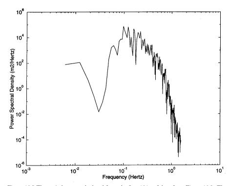
Figure 16.5 The periodogram calculated from the first 164 s of data from Figure 16.2. The Nyquist frequency is  $1.5625~{\rm Hz}.$
