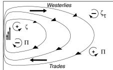
Figure 12.5 Conservation of potential vorticity can clarify why western boundary currents are necessary. Left: Vorticity input by the wind  $\zeta_{\tau}$  balances the change in potential vorticity  $\Pi$  in the east as the flow moves southward and f decreases; but the two do not balance in the west where  $\Pi$  must decrease as the flow moves northward and f increases. Right: Vorticity in the west is balanced by relative vorticity  $\zeta$  generated by shear in the western boundary current.
