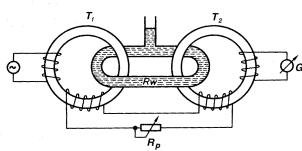
Figure 6.15 The induction method measurement of electrical conductivity uses a sea-water loop which couples two transformer loops  $T_1$  and  $T_2$ . The induced voltage in the second loop is proportional to conductivity  $R_w$  of the water. From Dietrich et al. 1980.
