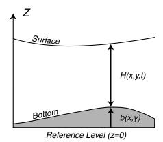
Figure 12.1 Sketch of fluid flow used for deriving conservation of potential vorticity (From Cushman-Roisin, 1994).
