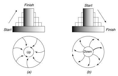
Figure 12.2 Sketch of the production of relative vorticity by the changes in the height of a fluid column. **Left:** vertical stretching reduces the moment of inertia of the column, causing it to spin faster; **Right:** vetical shrinking increases the moment of inertia of the column, causing it to spin slower (from von Arx, 1962).
