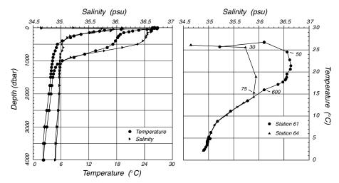
Figure 13.6 Temperature and salinity measured at hydrographic stations on either side of the Gulf Stream. Data are from Tables 10.2 and 10.4. **Left:** Temperature and salinity plotted as a function of depth. **Right:** The same data, but salinity is plotted as a function of temperature in a T-S plot. Notice that temperature and salinity are uniquely related below the mixed layer. A few depths are noted next to data points.
