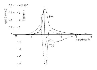
Figure 16.10 The function transfering wave energy from one part of the wave spectrum to another part via nonlinear wave-wave interactions T(n) where n is frequency. Dashed curve is for the theoretical spectrum  $\Phi(n)$ ,  $\times - \times$  is for a measured spectrum. The interactions extract energy from high frequency waves and transfer it to low frequency waves, causing the spectrum to change with time and generating waves going faster than the wind, (From Phillips, 1977: 139).
