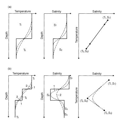
Figure 13.7 **Upper:** Mixing of two water masses produces a line on a T-S plot. **Lower:** Mixing among three water masses produces intersecting lines on a T-S plot, and the apex at the intersection is rounded by further mixing. From Tolmazin (1985).
