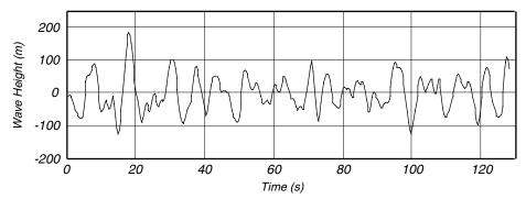
Figure 16.2 A short record of wave height measured by a wave buoy in the North Atlantic.
