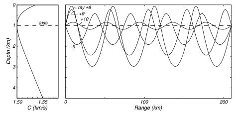
Figure 3.16 Ray paths of sound in the ocean for a source near the axis of the sound channel. (From Munk  $et\ al.\ 1995$ )
