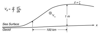
Figure 10.2 The slope of the sea surface relative to the geoid  $(\partial \zeta/\partial x)$  is directly related to surface geostrophic currents  $v_s$ . The slope of 1 meter per 100 kilometers (10  $\mu$ rad) is typical of strong currents.
