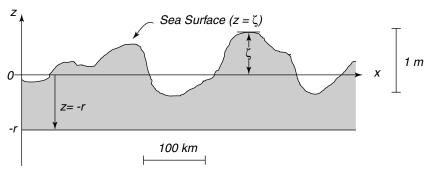
Figure 10.1 Sketch defining  $\zeta$  and r, used for calculating pressure just below the sea surface.
