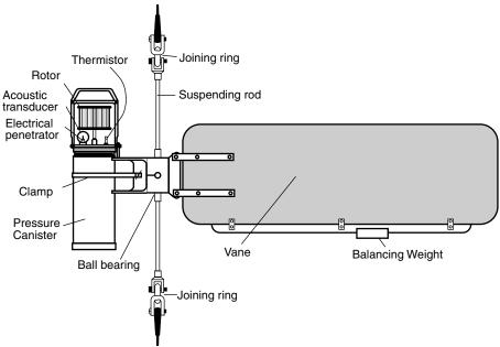
Figure 10.20 An example of a moored current meter with a Savonius roter to measure current speed, a vane to measure current direction, and a pressure-resistant housing for power and circuits to record the signal. The turns of the rotor are measured by the acoustic transducer. (From Dietrich, et al. 1980)
