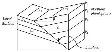
Figure 10.11 Inclination of the isobaric surfaces and interface between two homogeneous, moving water layers in the Northern Hemisphere.
