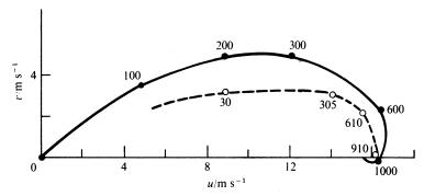
Figure 9.4 Ekman layer for the lowest kilometer in the atmosphere (solid line), together with wind velocity measured by Dobson (1914) - - - . The numbers give height above the surface in meters. The boundary layer at the bottom of the ocean has a similar shape. (From Houghton, 1977).
