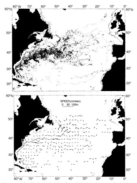
Figure 11.10 **Top** Tracks of 110 drifting buoys deployed in the western North Atlantic. **Botton** Mean velocity of currents in  $2^{\circ} \times 2^{\circ}$  boxes calculated from tracks above. Boxes with fewer than 40 observations were omitted. Length of arrow is proportional to speed. Maximum values are near 0.6 m/s in the Gulf Straem near  $37^{\circ}$ N  $71^{\circ}$ W. (From Richardson 1983).
