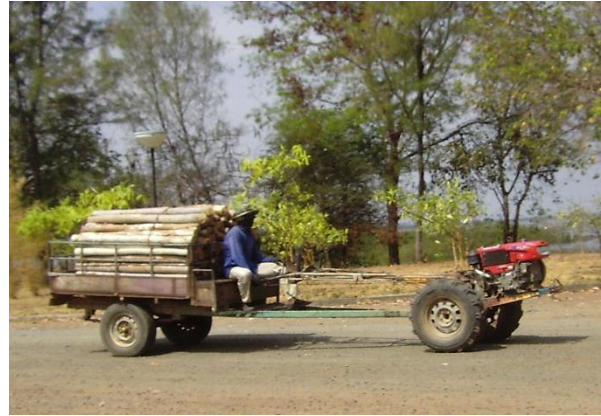
A Rot-E-Taek hauling logs in Isan, Thailand. This is one of many types of two-wheel tractor. Source: Wikipedia
