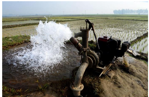
A diesel-powered shallow tubewell irrigates rice seedlings in Jamalpur, northern Bangladesh Source: Mamunur Rashid / Alamy).
