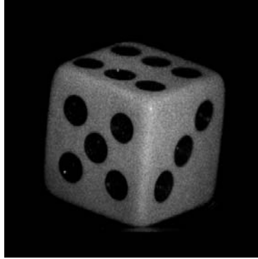
Figure 9. Image of a 3D object obtained by phase-shift interferometry with the optical system in Fig. 8.
