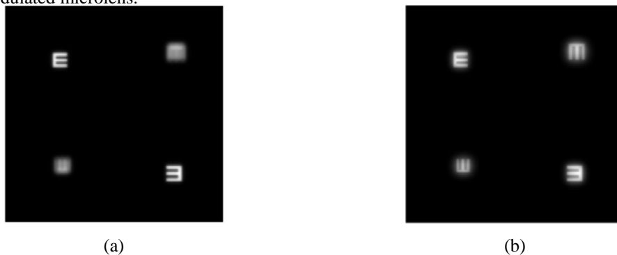
Figure 3. One of the elemental images captured with: (a) a conventional microlens array and (b) an amplitude-modulated microlens array. The 3D scene object contains tumbling charts located at different distances.
