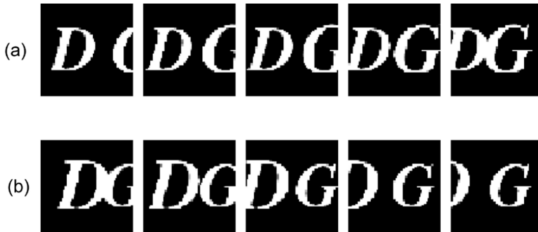
Fig. 12 (a) Real, pseudoscopic image calculated from the elemental images in Fig. 11(a); (b) Real orthoscopic image calculated from the elemental images in Fig. 11(b). In both reconstructions we assume that the observer is placed at 500 mm from the microlenses, and he/she laterally displaces the eye from left to right. The eye displacement is from x=-25\text{mm} to x=+25\text{mm} .
