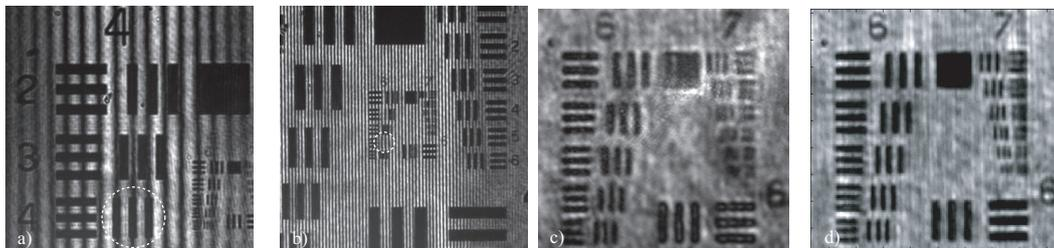
**Figure 1.** Experimental results for the the tunable-frequency SI microscope: (i) Illuminated target for two different axial locations of the biprism; the dashed circles correspond to the groups in the target with: (a) 22 lp/mm; (b) 102 lp/mm. (ii) Images of the central region of the target: (c) Original brightfield setup; (d) SI synthetic image with the illumination pattern in (b).
