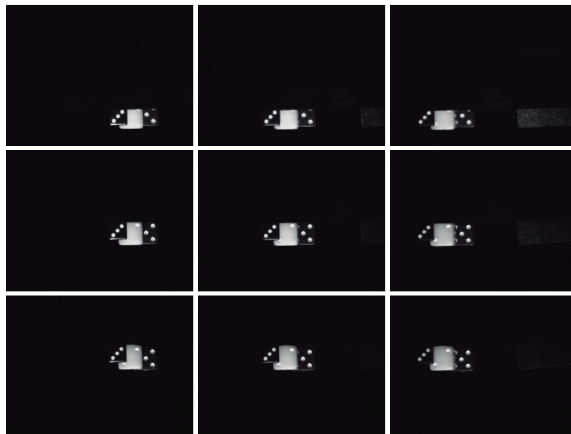
Fig. 4. Elemental images corresponding to positions: (2,1), (2,6), (2,11), (6,1), (6,6), (6,11), (9,1), (9,6), and (9,11), for \lambda = 650\text{nm} .
