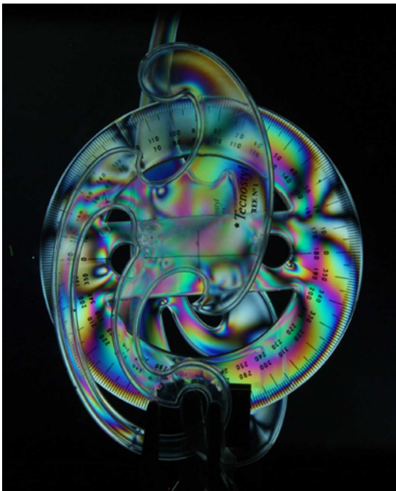
Fig. 11. Set of drawing tools, having mutual occlusions, under the analysis of a conventional 2D polariscope.
