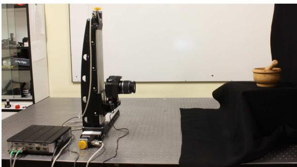
Fig. 7. Experimental setup for capturing different EIs of a 3D object. The mortar is located inside the training volume of the fuzzy system.
