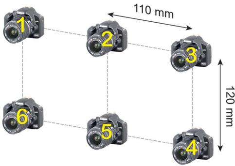
Fig. 5. Camera arrangement used for calibrating the fuzzy system and for capturing the information of a 3D scene.
