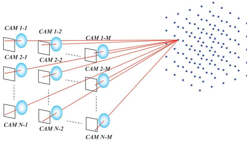
Fig. 1. Array on  $N \times M$  cameras capturing a cloud of points whose 3D coordinates are known.
