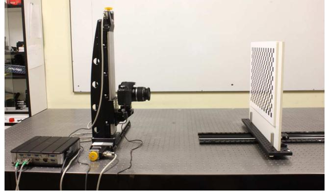
Fig. 4. SAIL setup for capturing different perspectives of the checkerboard pattern employed during the calibration process.
