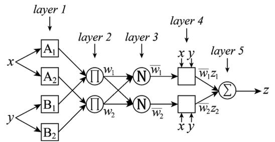
Fig. 2. ANFIS architecture of a fuzzy system with two inputs and with two rules.
