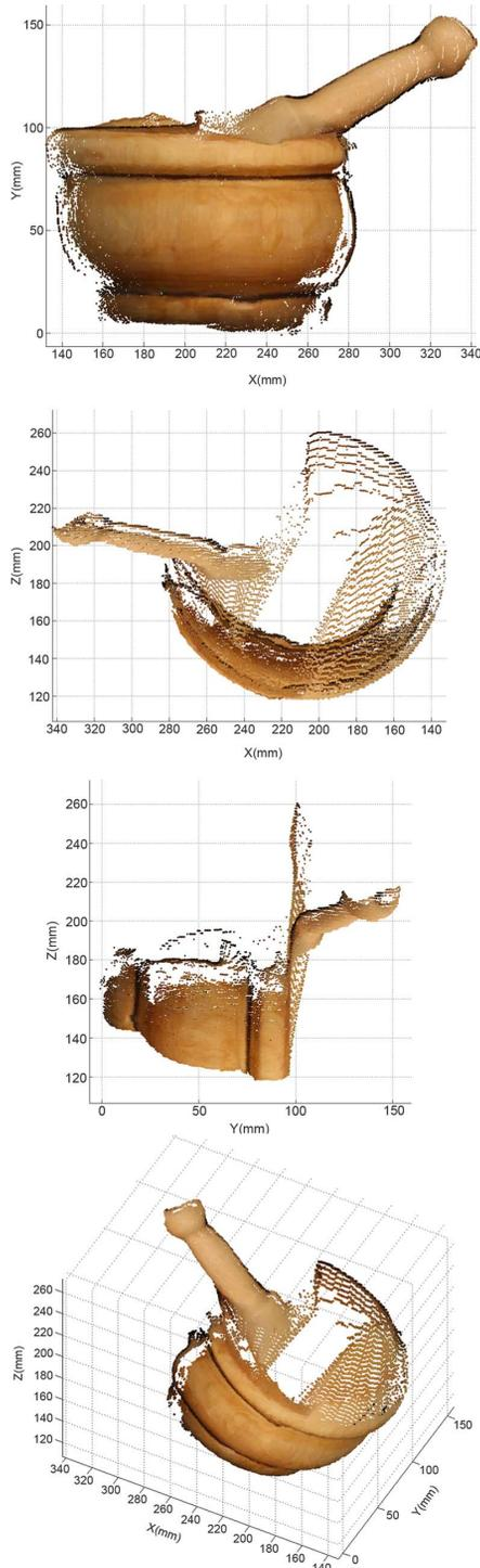
Fig. 10. Computational reconstructions of the mortar rendered from different perspectives. The fuzzy system has been calibrated using camera positions 1, 3, 4 and 6.
