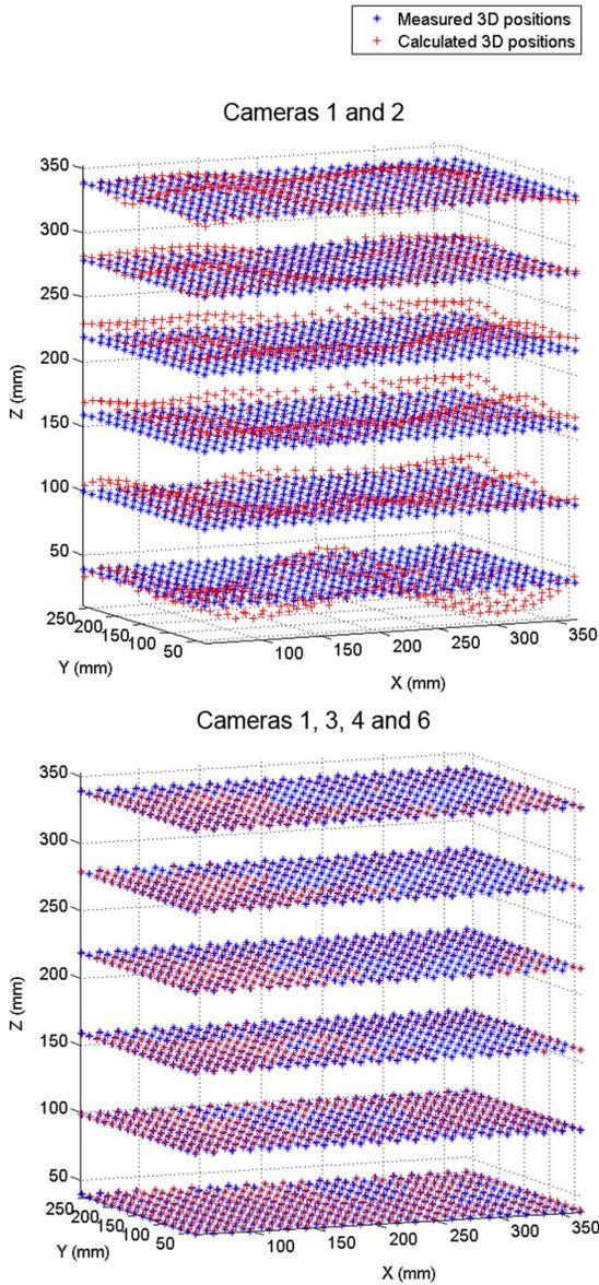
Fig. 6. Computational reconstruction of the cloud of points defined by the checkerboard B for six different axial positions inside the training volume. Reconstructed points are compared with the measured positions of those points.
