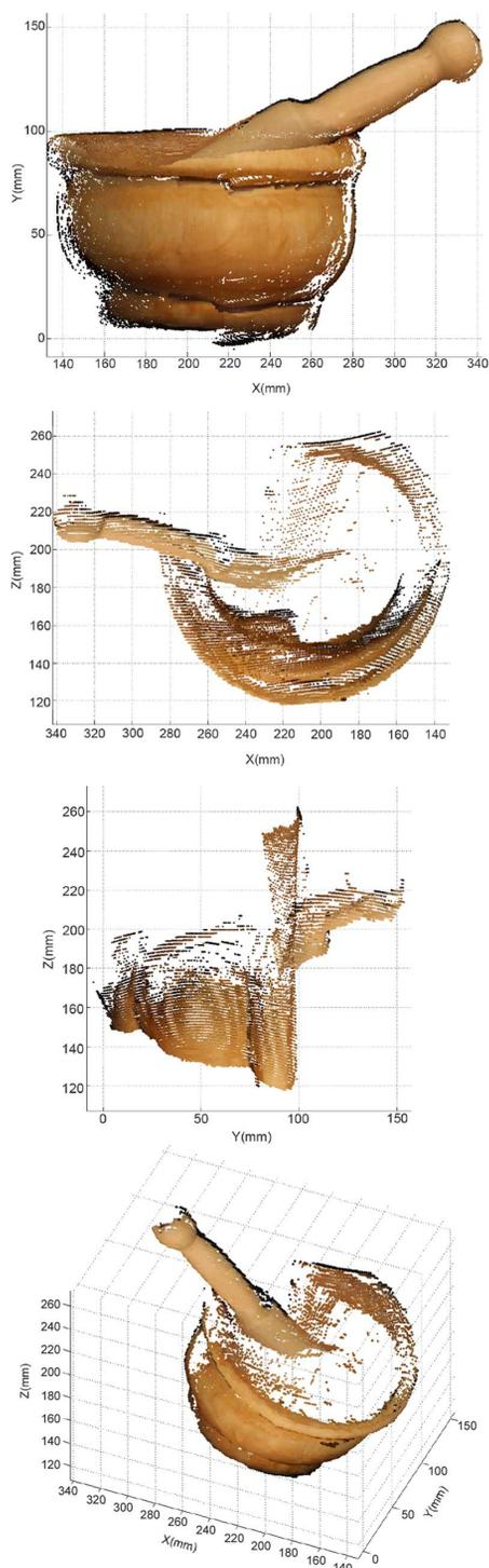
Fig. 12. Computational reconstructions of the mortar rendered from different perspectives. The fuzzy system has been calibrated using camera positions 1 and 2.
