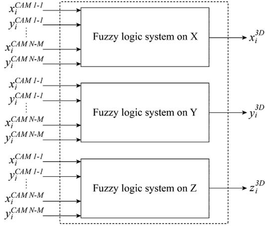
Fig. 3. Implicit camera calibration scheme based on our fuzzy model.
