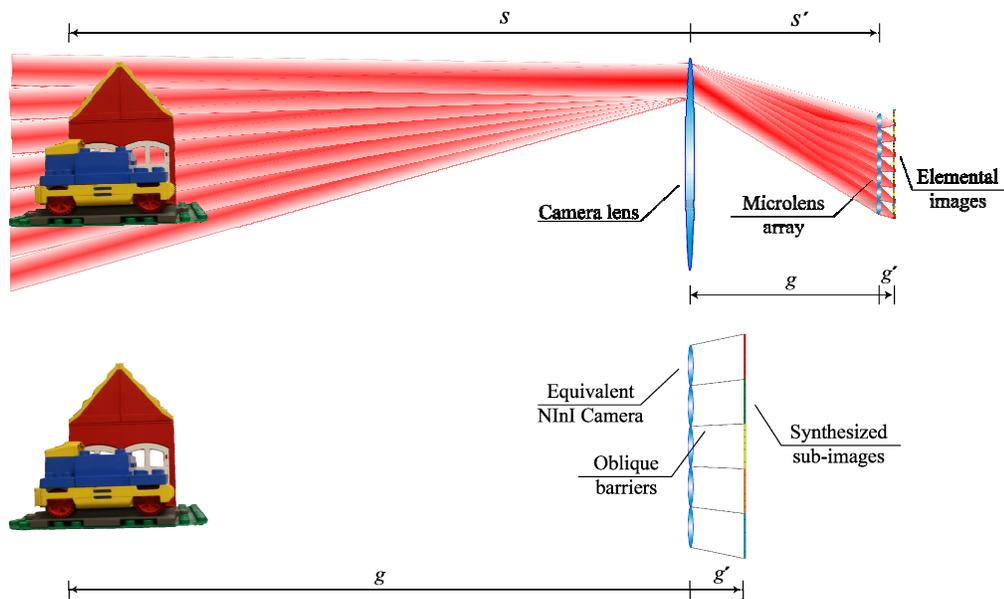
**Figure 2** Subimages of a plenoptic camera. Note that they are equivalent to the elemental images of an integral imaging system when the lenses are placed in the main lens plane.
