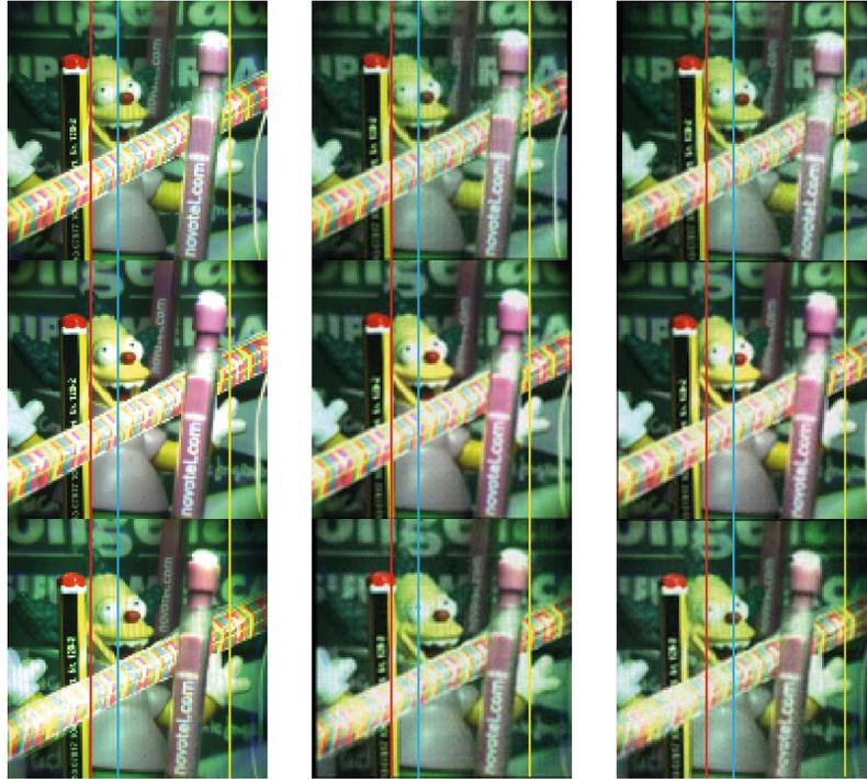
**Figure 6** Computer reconstruction of the visualization process. Each column of images corresponds with one set of views obtained from the plenoptic image shown in Figure 4 and Figure 5. In each set of images, three lines have been plotted to highlight the invariance of the reference plane.
