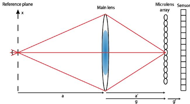
**Figure 1** Diagram of a plenoptic camera.
