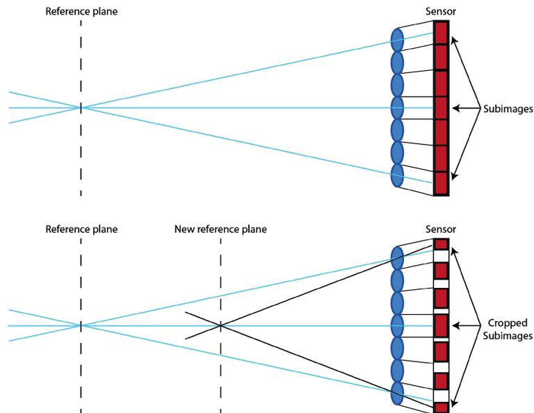
**Figure 3** Illustration of how the position of the reference plane is moved in plenoptic systems.
