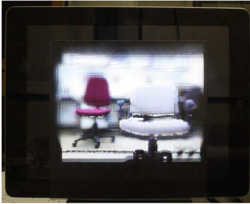
Fig. 6. Single-frame excerpt from video recording of the implemented InI monitor (Media 1). The video is composed of views of the monitor obtained from different horizontal and vertical positions.
