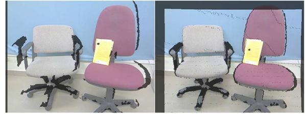
Fig. 1. (left) Raw mapping result and (right) reconstructed mapping result after our proposal method. See text for further details.
