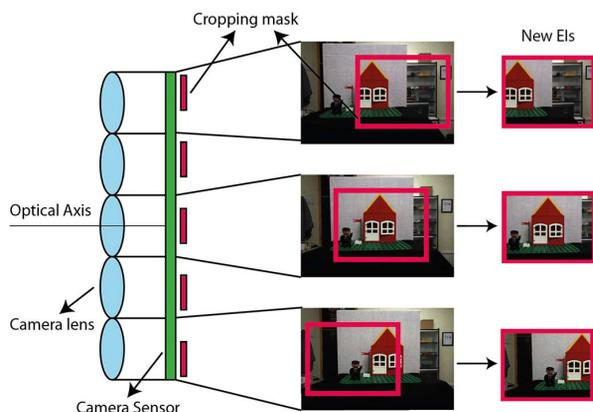
Fig. 1. Illustration of the cropping procedure. Note that the position of the cropping mask depends on the relative position of the EI in the integral photography. After cropping, a new set of EIs is generated.
