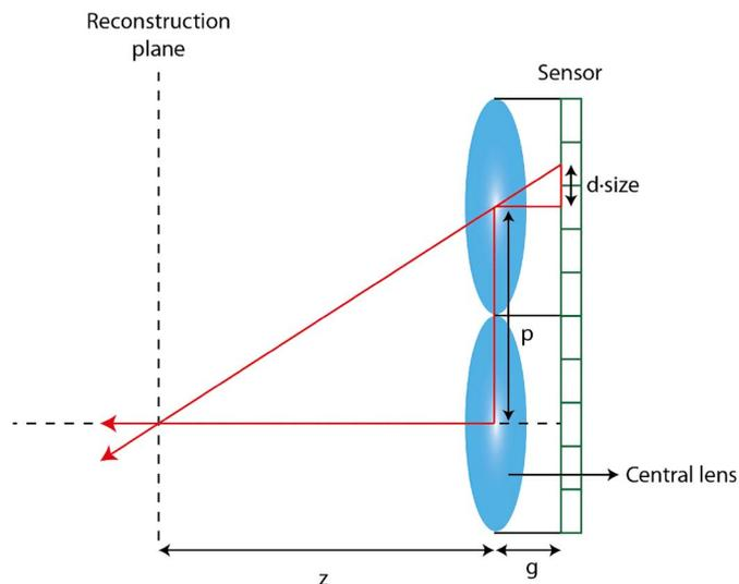
Fig. 2. Relation between the shift in pixels of the cropping mask and the reference plane. In the figure,  $d$  is the shift in pixels,  $g$  is the gap between lens and sensor, and  $p$  is the pitch of the lenses or the axial separation between cameras and size is the size of the pixels.
