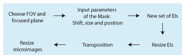
Fig. 3. Workflow diagram of the SPOC 2.0 algorithm: 1. Choose FOV and focused plane, 2. Input the parameters of the cropping mask, 3. Apply the mask, 4. Resize the new EIs, 5. Apply transposition, 6. Resize microimages.
