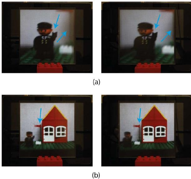
Fig. 10. Frames of the movie obtained by recording the IP monitor from a given distance, 50 cm, but changing the viewing angle: (a) the FOV and reference plane is centered at the doll. (b) the FOV shows the whole scene and the reference plane is at the house plane. In both cases, there are two images that show the end left and the end right views respectively and arrows pointing the parallax differences. The movie is shown in MEDIA2.
