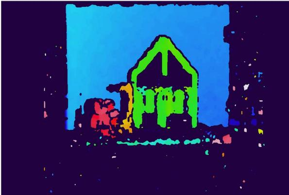
Fig. 5. Disparity map obtained from two EIs of the integral photography using the SAD method. It is possible to distinguish different objects of the scene. In addition, knowing the parameters of the capture permits to obtain the depth information of the scene.
