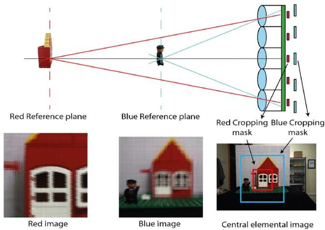
Fig. 4. Illustration to show how the change of the size and position of the cropping mask in each elemental image modifies the FOV and the reference plane. The more the cropping mask is separated from the center of the EIs the closer the position of the reference plane is (see the red and blue cropping mask examples).
