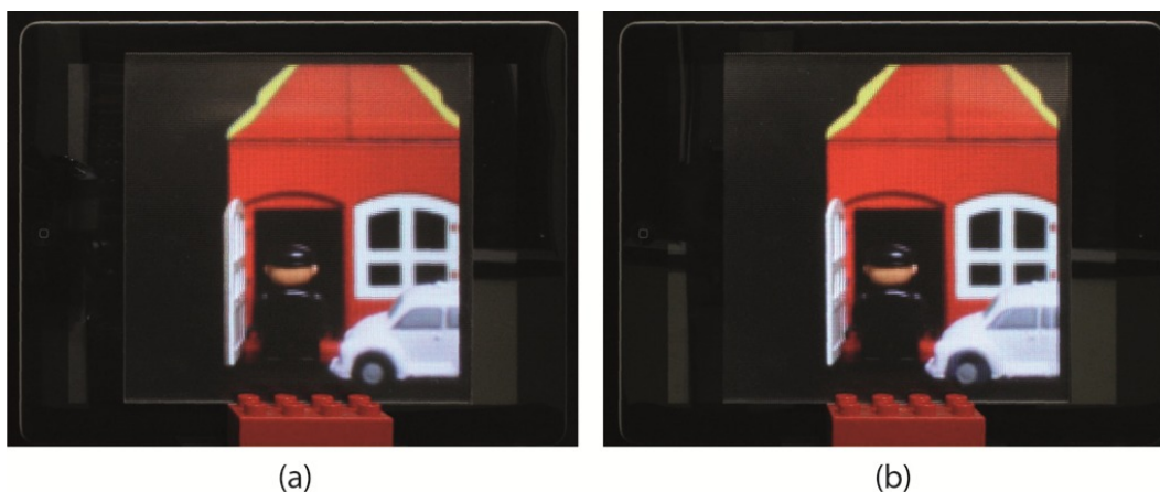
Figure 7. Two photos of the InI monitor displaying the same frame of the 3D movie. Each photo was taken from two different position to simulate the movement of an observer viewing the InI monitor and moving the head from left to right. (a) Shows the view from the left and (b) the view from the right.
