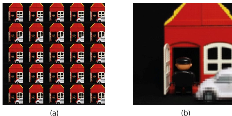
Figure 1. (a) Set of 5x5 elemental images from an 11x11 integral image. (b) Plenoptic image generated from the integral image shown in (a).
