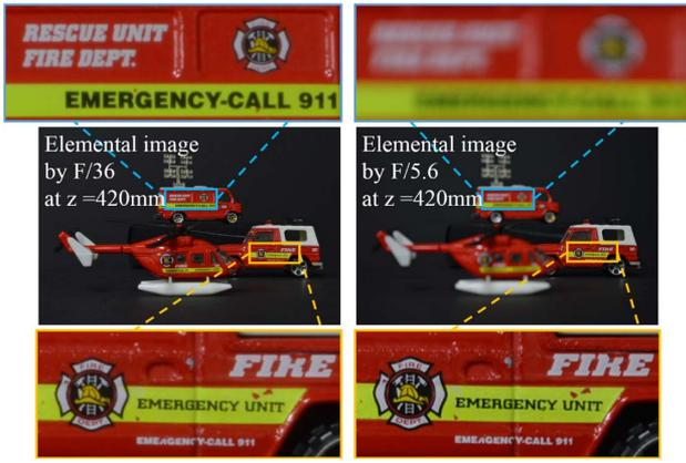
**Fig. 10.** Comparison between elemental images by  $f/36$  (left) and  $f/5.6$  (right) at a distance of 420 mm.
