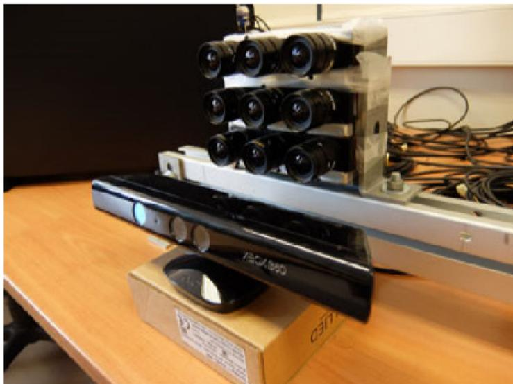
Two-sensor setup used in the experiments:  $3 \times 3$  camera array on top and Kinect device below. (Reprinted from [8].)
